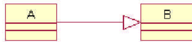
Figure 7.2 - UML representation for Inheritance. A inherits from B or A is-a B.
