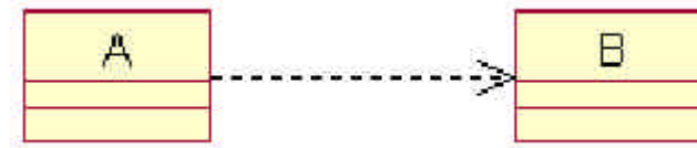
Figure 7.6 - UML representation of Dependency. A depends-on B.
