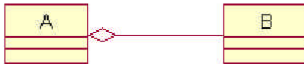
Figure 7.10 - UML representation of Aggregation. A contains B or A has-a B.
