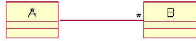
Figure 7.8 - UML representation for Multiplicity. A is associated to-many B.
