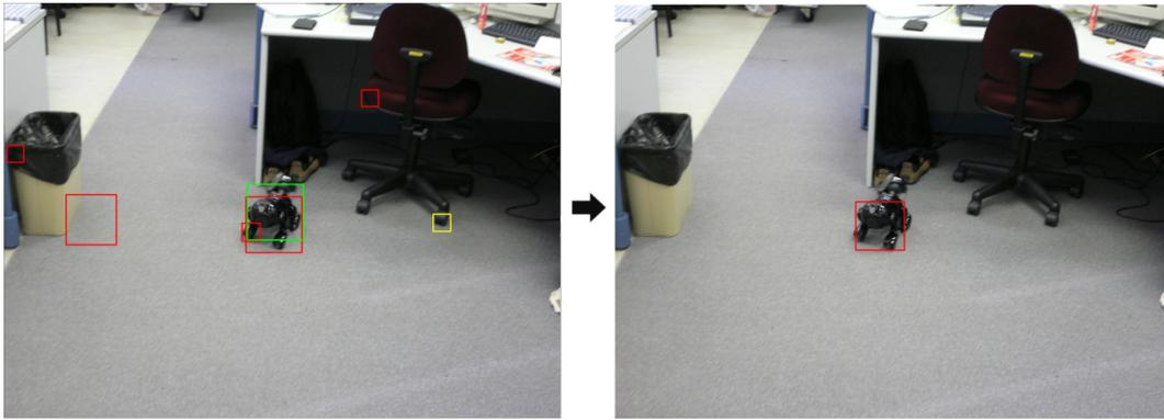
Fig. 6. Example of the Classifier Voting. On the left, various classifiers (using different colours) detect the AIBO in multiple locations. Voting is applied to these regions to find a common consensus. The resulting single region is shown on the right.
