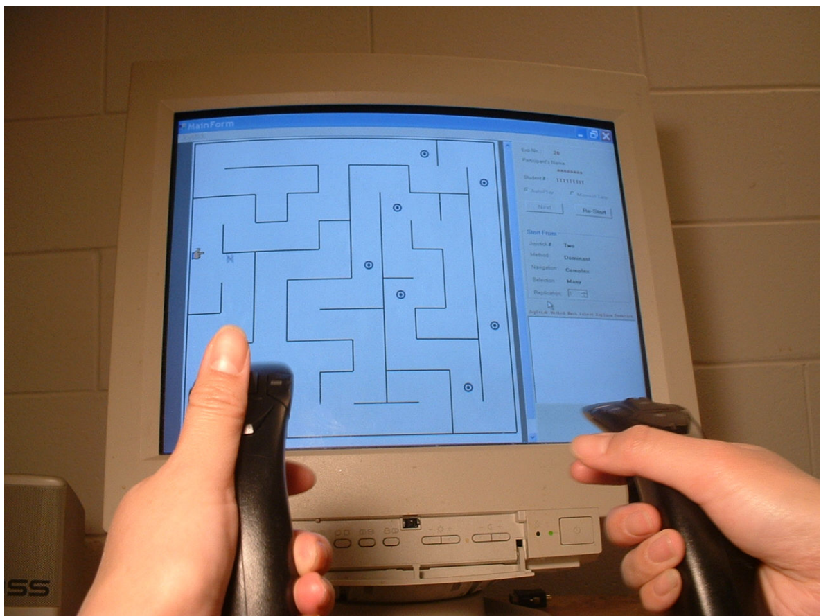
Figure 5: Experimental setup in experiments 1 and 2 where the user has two joysticks, one for the task of navigation and the other for selection.
