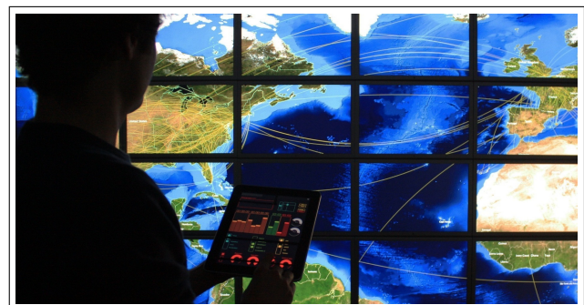
Figure 1. Interacting with a wall display using a tablet that features both an area dedicated to high-precision pointing for the remote selection of graphical objects on the wall, and control widgets to act on those objects.
