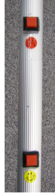
Figure 2 – Broomstick buttons for triggering happy or sad sounds.
