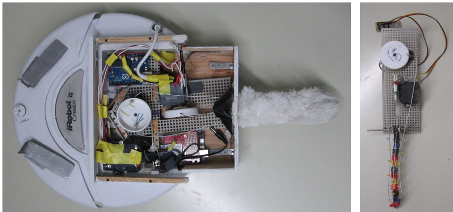
Fig. 3. Top-view of the tail assembly and before putting it inside the wooden box (right).
