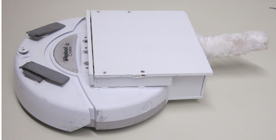
Fig. 2. An iRobot Create with our dog-tail attached.
