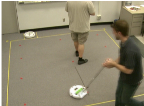
(a) Authoring interactive robot locomotion style using the broomstick, showing a Roomba reactor how to interact with a person leader.
