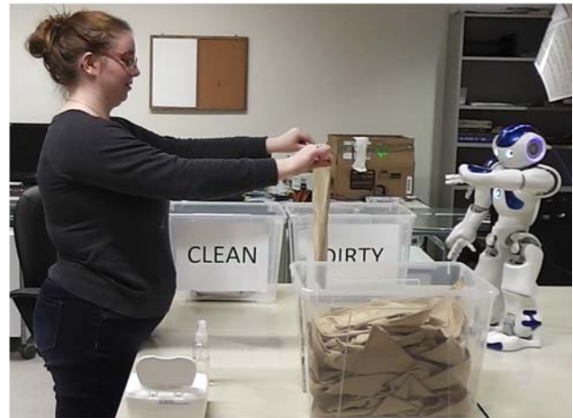
Figure 2. A participant and a robot working collaboratively to sort pieces of cloth. The participant holds up a piece and the robot scans it, then indicates that dirt is detected on the top left corner with pointing and verbal feedback.
