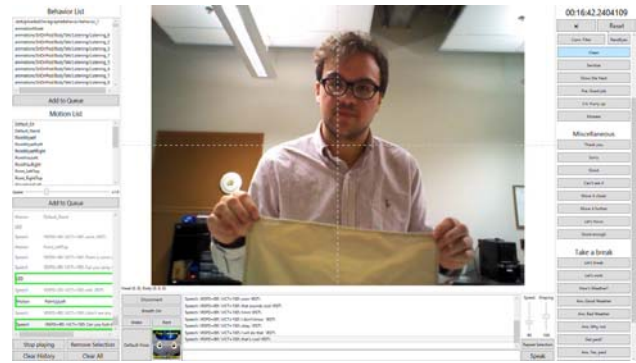
Figure 5. Our in-house Wizard of Oz interface used during the experiment. The various panels and buttons enable the operator to activate a range of pre-defined behaviors, gestures, conversation topics, etc. The operator can also give low-level commands and custom speech for unexpected behavior. Here, the participant is nodding his head when the robot says the piece of cloth is clean.
