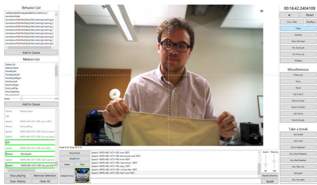
Fig. 3 Our Wizard of Oz interface used during the experiment. The various panels and buttons enable the operator to activate a range of pre-defined behaviors, gestures, conversation topics, etc. The operator can also give low-level commands and custom speech for unexpected behavior. Here, the participant is nodding his head when the robot says the piece of cloth is clean
