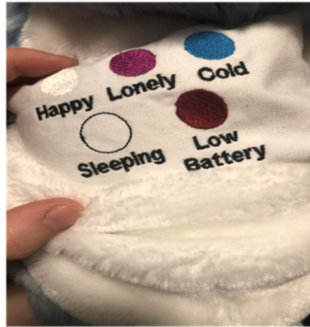
Figure 4. In addition to making the robot feel comfortable to hold, the embroidered heat pack reminds people what the horn colours mean
