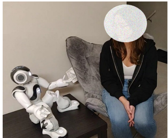
Figure 1. Our conversational robot design uses well timed simple questions and prompts to encourage people to self-reflect, aiming to support well-being without needing the robot to parse or understand what the user says. (re-created interaction. participants were not recorded).
