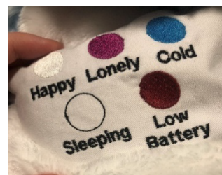
Figure 3: Embroidered heat pad explains the horn colours and warms the robot.
