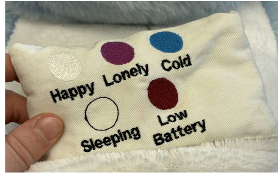
Figure 2: Embroidered heat pad explains the horn colours and warms the robot.
