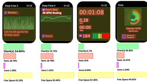
Figure 2: Space usage analysis on four illustrative visualization interfaces across two applications <sup>2</sup>indicating the percentage of free space and of space occupied by each visual element: charts, texts and icons.
