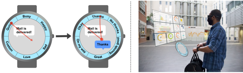
Fig. 13. In a (left) we demonstrate quick replies utilizing B2B and marking menu responses. In b (right) we demonstrate how B2B on a smartwatch could be used in AR. Note, the interaction could be eyes-free of the actual smartwatch while controls are displayed within the virtual content.
