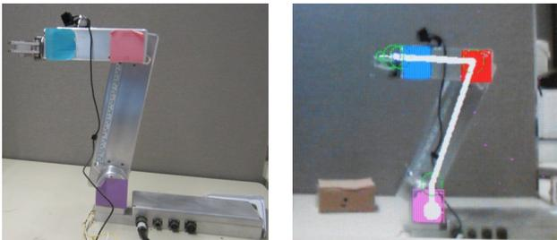
Figure 6. Arm tracking using simple computer vision, required to provide current-configuration state feedback to the user
