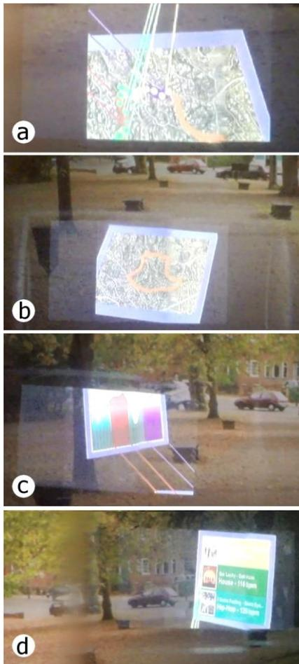
Figure 6. Images of our implementation, through a Moverio BT-100 HWD. The spatial UI assists the user in gaining insight from interspatial links (a) between a map (b), a heart rate chart (c), and a song playlist (d).
