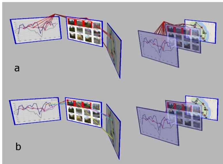
Figure 9. Interspatial visual links can join a set of data points belonging to a group selection (a). Different coloured links can show relations across views while contrasting between different selections (b).
