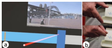
Figure 6: Demo #3 uses bimanual input to simultaneously specify a position on a film clip (a), and crop using a “snipping” microgesture (b).
