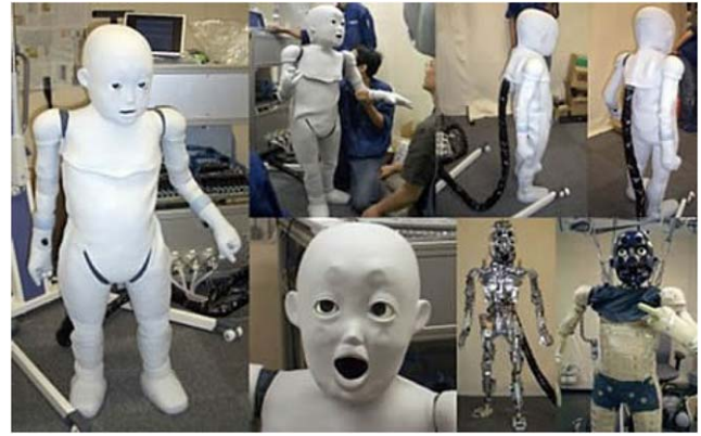
(a) CB^2 baby robot, developed by the JST ERATO Asada Synergistic Intelligence Project [40]
