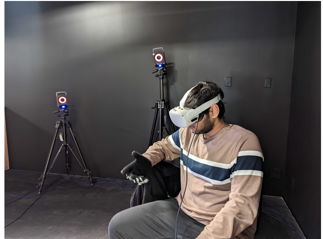
Figure 2: The setup used to demonstrate the example applications during the study. We used a Oculus Quest 2 HMD with a Unity application being executed with Oculus Link. A Vicon motion tracking system was used to track the motion of the HDM and the hands with optical markers.
