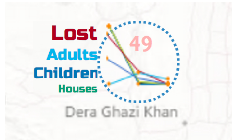
Figure 10: An early version of the main component of Geo-Temporal Tag Visualization showing the frequency of words listed on the left. The number in the center shows the number of reports received in that time period.
