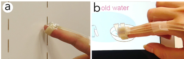
Figure 11: Example scenarios using mixed-reality haptics to add feedback to existing objects and devices. a) a user moves their finger over a wall, and feels vibration feedback as her hand passes over wiring hidden behind the wall. b) a user touches an interactive children's book, which provides thermal feedback corresponding to the on-screen content.
