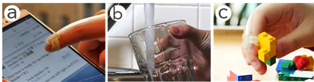
Figure 10: Sample scenarios where mixed-reality haptics could be used; a) while operating existing technology b) performing activities in wet or dirty environments c) performing activities that require manual dexterity.
