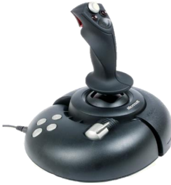
Figure 3. The joystick we used for tangible priming – Microsoft Sidewinder Force Feedback 2 USB joystick. It can be dynamically programmed to have different stiffness settings.
