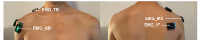
Figure 3: EMG sensors placement of four investigated muscles that contribute to shoulder range of motion.
