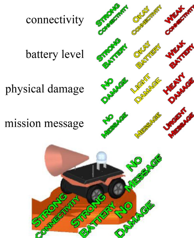
Fig. 3 Text representations for all states conveyed. Each state consists of two words: a noun and descriptive adjective. Text is tilted to maximize size within a square space, and we used a black outline to increase contrast and maximize visibility
