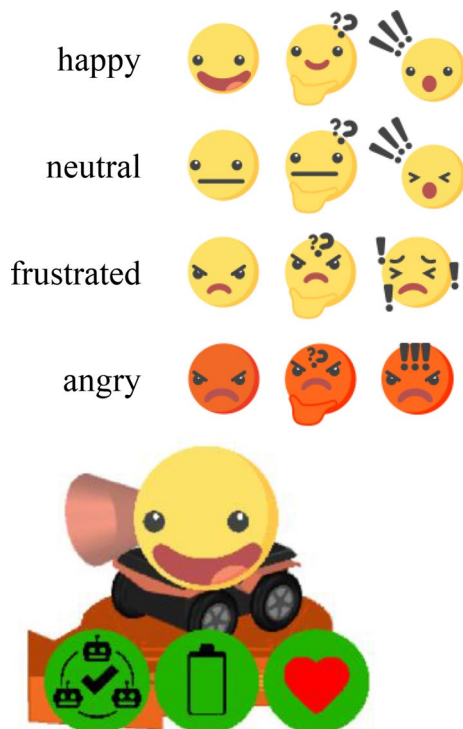
Fig. 5 The emoji uses facial expressions to represent general states. The left faces above are for no message, the middle faces for message available, and right faces for urgent messages
