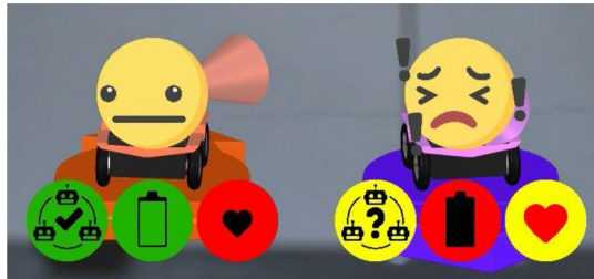
Fig. 8 Our team state representations for two team robots with emotional information encoding. Note that the message state is superimposed on the face
