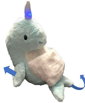
Figure 2. SnuggleBot’s embedded hardware provides feedback: its tail can move up and down, flippers can wiggle, and its horn can glow a range of colours.
