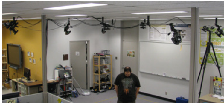
(b) ceiling-mounted vicon cameras
