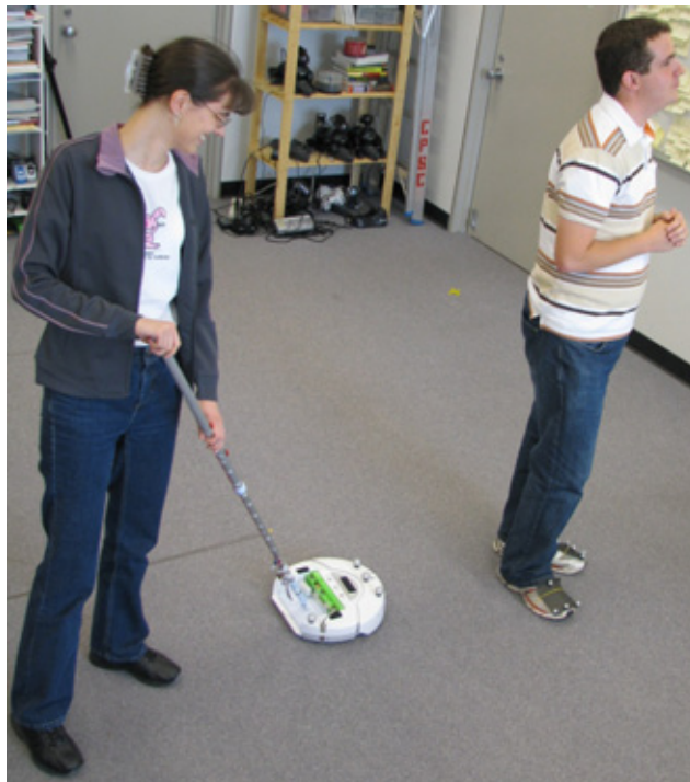
Figure 1.4: demonstrating to a robot using our puppet master interface the social style of how it should interact with a person
