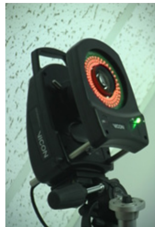
(b) Vicon MX-F40 camera with infrared emitter
