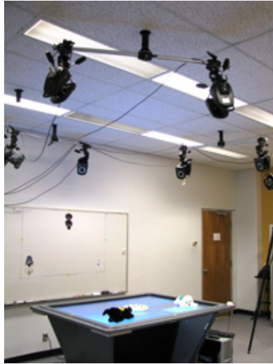
(a) the tabletop workspace with tracking cameras
