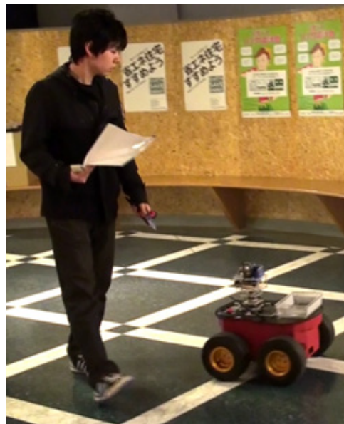
Figure 4.4: a robot being led on a leash from behind, where the person stays behind the robot
