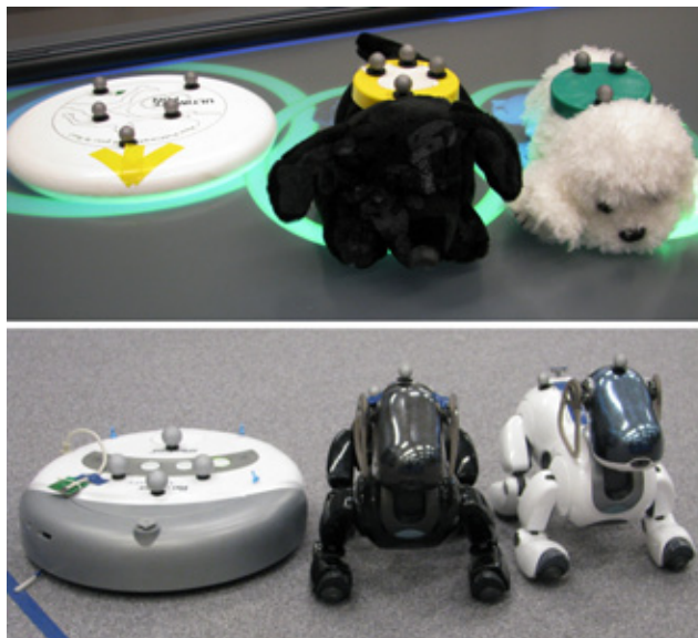
Figure 5.3: our TUIs and corresponding robots, two Sony AIBOs and an iRobot Roomba
