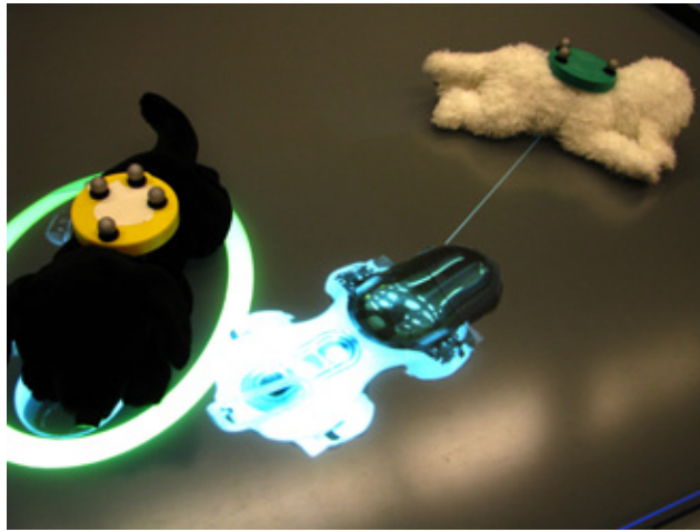
Figure 5.2: touch and toys interface details: the black Sony AIBO dog is at its target location, shown by the green halo, and the white AIBO is on its way to its location, shown by the graphic and line
