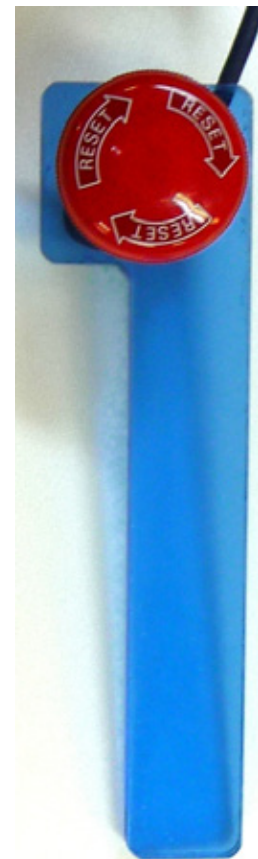
(b) close-up of the leash handle, with the red emergency-stop button
