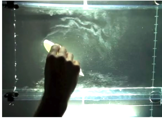
Fig. 6: A water tunnel visualization where a wing model can be rotated to examine the impact of orientation on aerodynamism [31]. Here the physical referent is the wing and the physical presentation is the set of water bubbles.
