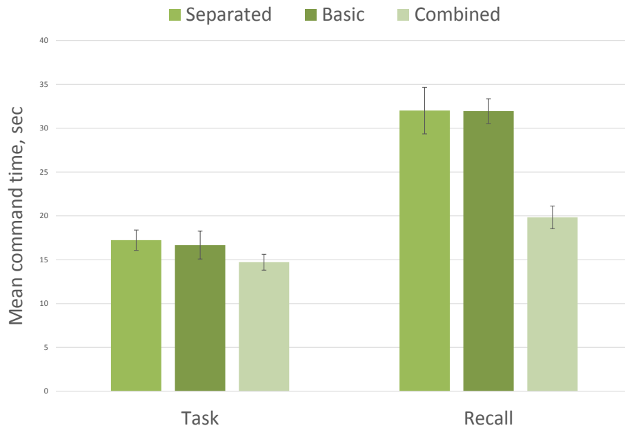
Figure 5.2: Mean selection time between commands (with standard errors) for the main task (left) and the recall task (right)
