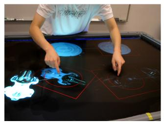
Figure 4. A user simultaneously interacting with two robots. Touching inside the circle does a translate, touching outside the circle (but inside the square) performs an RNT operation.
