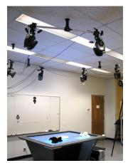
(a) The tabletop workspace with the TUIs on top and the Vicon ceiling setup.
