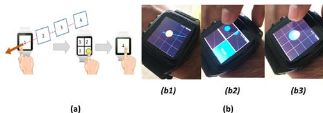
Figure 12: (a) FlickPan. (b1) Initial screen. User flicks. (b2) Thumbnails of next screens (in the flick direction) appear. (b3) Selected thumbnail is now the current screen.
