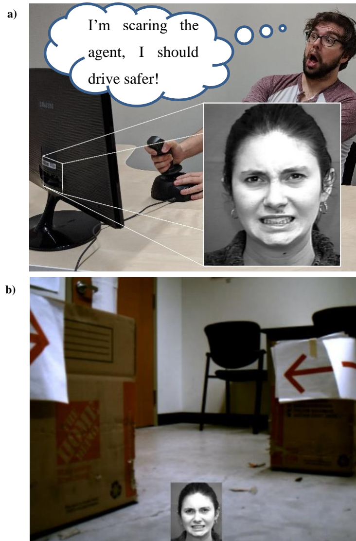
Figure 1.4. a) An on-screen “virtual passenger” agent reacts to poor driving by exhibiting anxiety, with the intention of impacting the teleoperation experience. b) the interface displayed during robot teleoperation.
