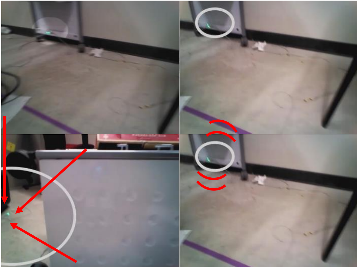
Figure 3.5. Our four interfaces for the first design iteration: dark (top-left), circle (top-right), target (bottom-left), bounce (bottom-right). Red markup indicates motion and are not shown in the interface.
