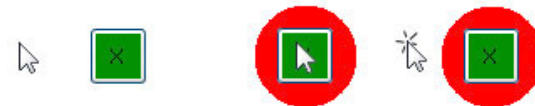
Figure 2. Target Lock technique walkthrough: (1) User moves the pointer toward a target. (2) Moving the pointer over the target highlights the target. (3) Clicking the left mouse button selects the highlighted target.
