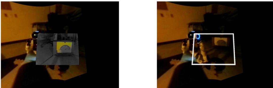
Fig. 2. Monocle detail-in-context interface. the sharp-view (left) integrates into the wide view; (right) the monocle toggled off by the operator. Third-person view provides wide context but at a reduced clarity due to limited resolution. The first-person view has a narrow field-of-view to provides more clarity.
