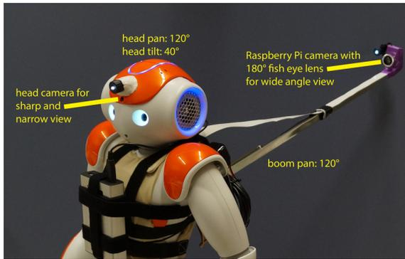
Fig. 3. Robot with boom; boom camera is above the robot, pointed downward to capture the full body. Both cameras have LED lights attached to aid in dark environments.
