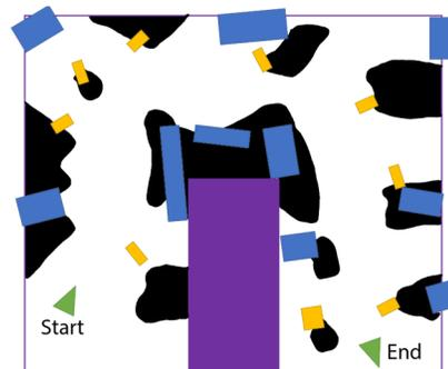
Fig. 5. USAR evaluation environment picture and map. The robot is at the start position. Blue: equipment. Yellow: rubble. Black: (fake) holes. Purple: wall.
