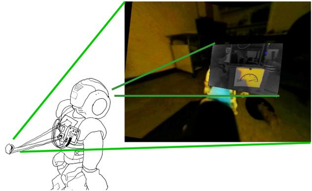
Fig. 1. *Monocle*, a fully interactive detail-in-context teleoperation interface with wide pannable (behind robot) and narrow pan-and-tilt (in robot head) views. An operator can move the monocle around to gain detail where needed. (Low light, image quality due to search and rescue scenario).
