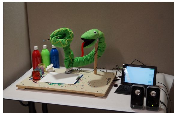
Figure 2. Picasssnake, the painting robot, is ready to draw an abstract painting. The robot is connected to a laptop to process audio input: MP3 file, audio loopback, or microphone.
