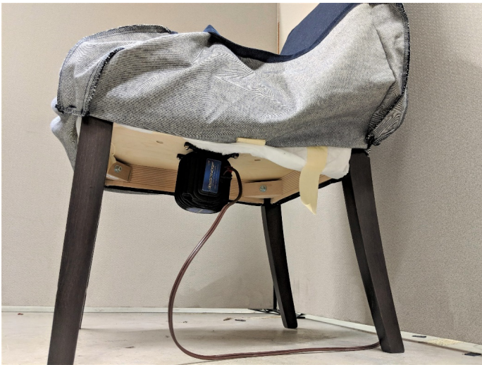
Fig. 2. The vibration motor (Buttkicker Low Frequency Effect Transducer) mounted to an Ikea chair. The chair skirt is lowered to conceal the equipment and wires from participants.
