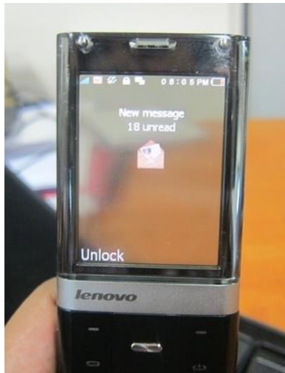
Figure 6: T-OLED used in this thesis is the screen of Lenovo S800 mobile phone [14]
